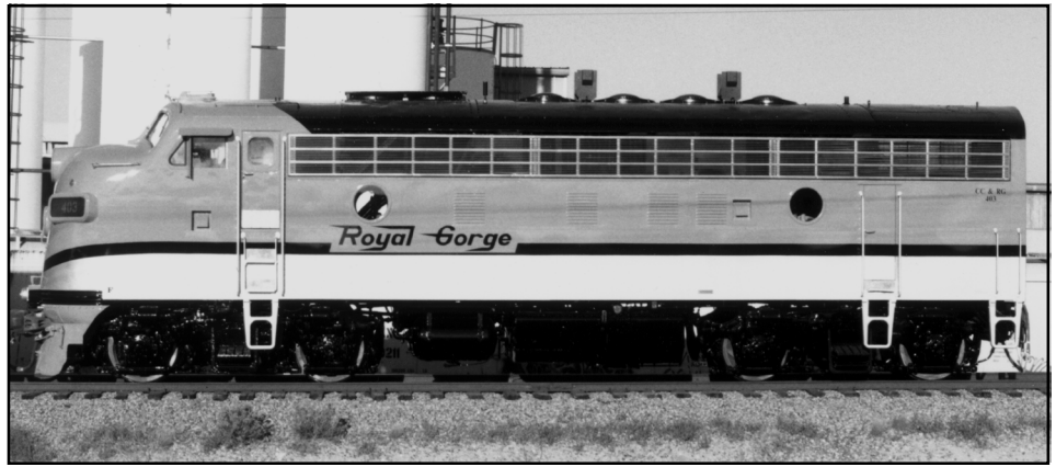
Cañon City & Royal Gorge's F-7A #403 looks sharp in its Rio Grande inspired scheme in early October, 1998. Painters Jim Webb and Lennie Miles of Liberty Railway Services, Inc., of Pueblo, CO, applied Imron and a clear coat to keep this F-unit looking sharp for years to come.
